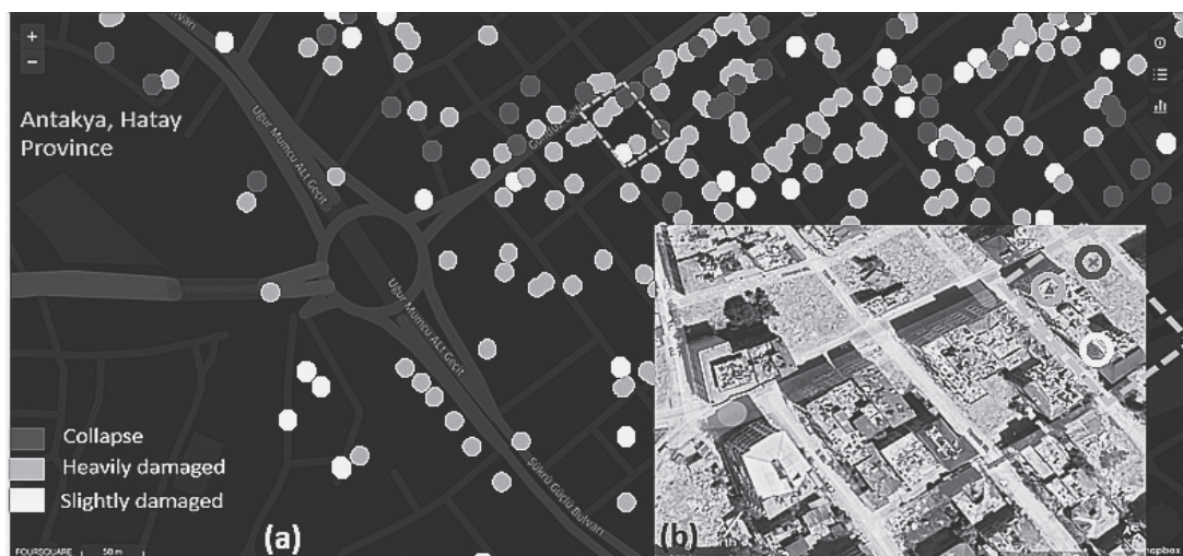
Figure 1. Example of the identified location of houses and damage levels considered in Hatay (Close-up view).
